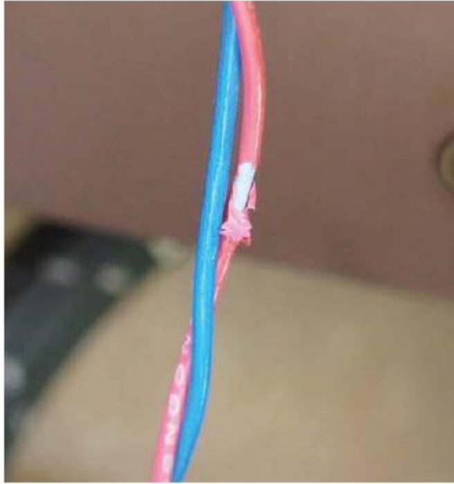
Damaged first officer oxygen light plate 5 volt AC wiring on a different 777-200 airplane
